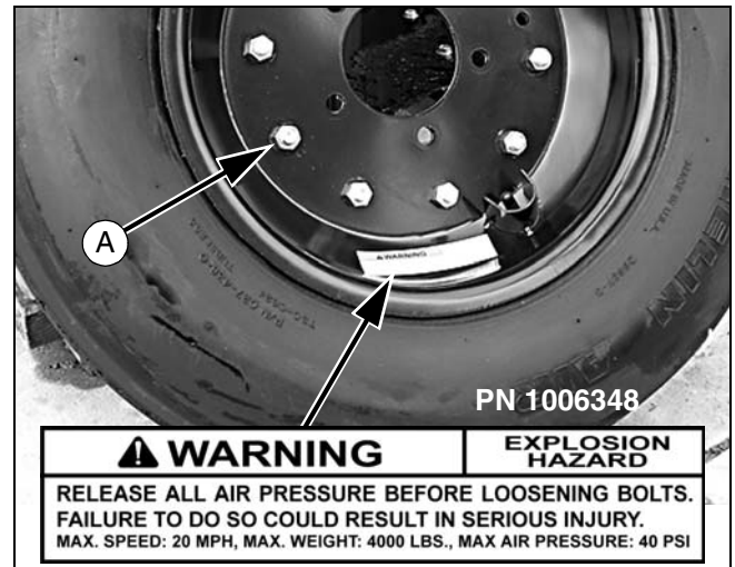
Figure 9. Split Rim Tire Servicing
